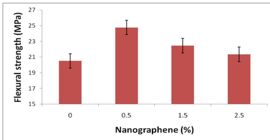
**Fig 1: Nanographene loading vs. flexural strength of FPF/HDPE nanocomposite**
