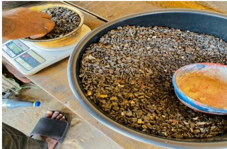
**Plate 4: Recycled/crushed polyethylene (HDPE)**
