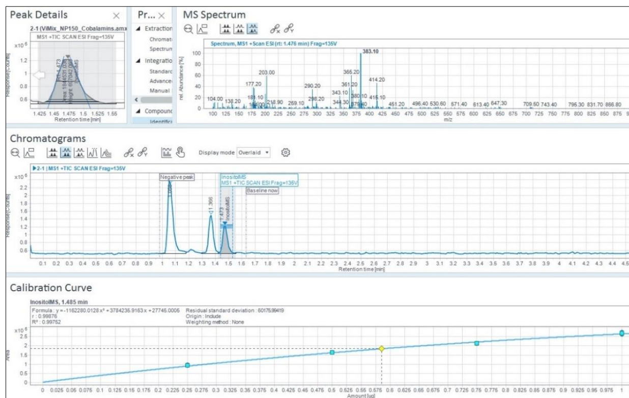
Figure 7: Analysis of inositol in a multicomponent injection solution. Data processing screenshot
