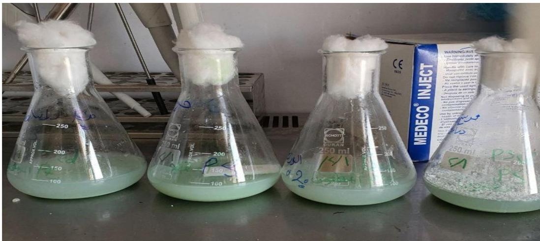
**Figure 3: Polyethylene inoculation with bacteria**
