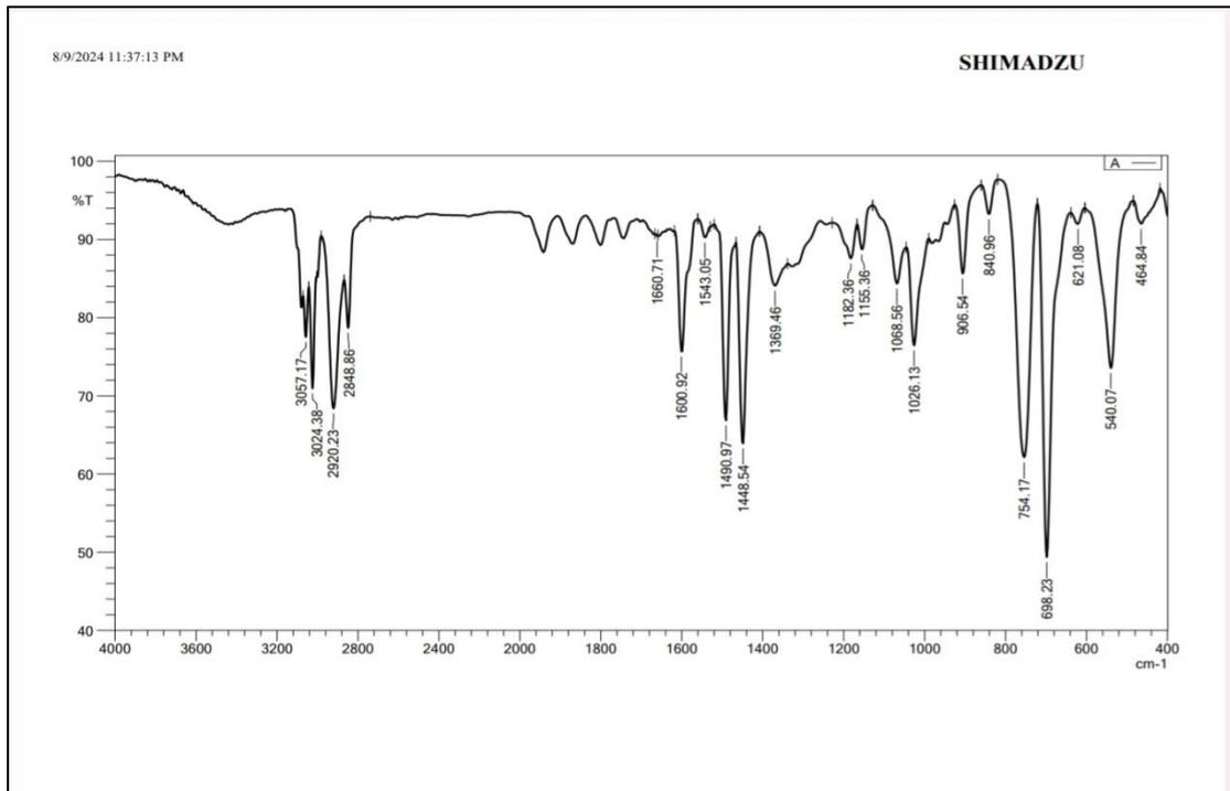
**Figure 4a: FTIR spectra of polyethylene (PE) before consumption by bacteria**
