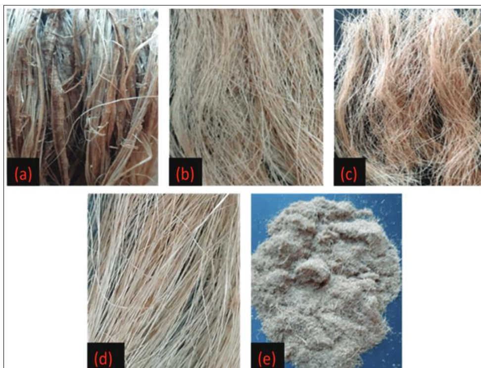
Figure 3: photographic images of; (a)untreated dry banana pseudo-stem(BPS), (b)banana fiber extracted through alkali treatment method, (c)banana fiber extracted through acid treatment method, (d)banana fiber extracted through emulsion treatment method, (e)adhere lignin by-product of emulsion treatment process(Bar et al. , 2022)
