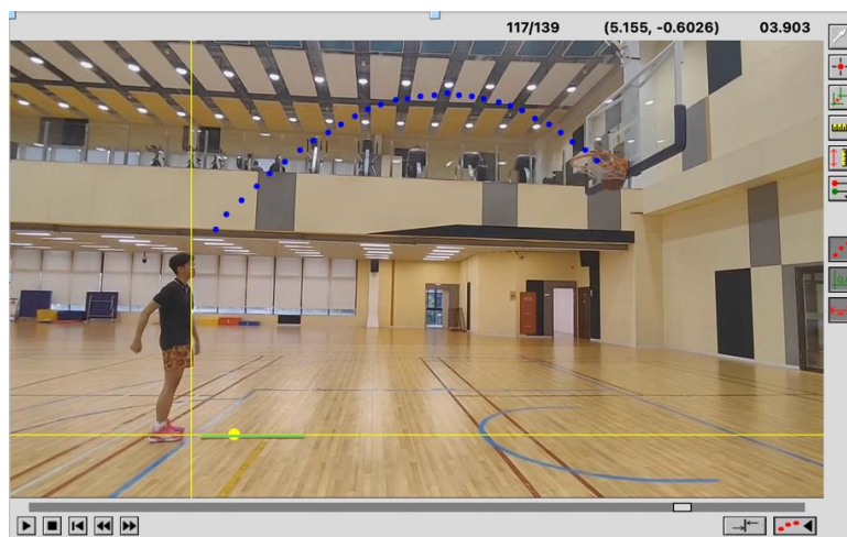
Figure 2: Video analysis set-up. The mutually perpendicular yellow lines represent the 2-D coordinate of the scene, and the green lines represents the calibration for the scene, which represent this amount of length corresponds 1 meter in the real life. The uninterrupted blue dots represent the basketball's track, and the realistic track equations that logger pro created is based on this track
