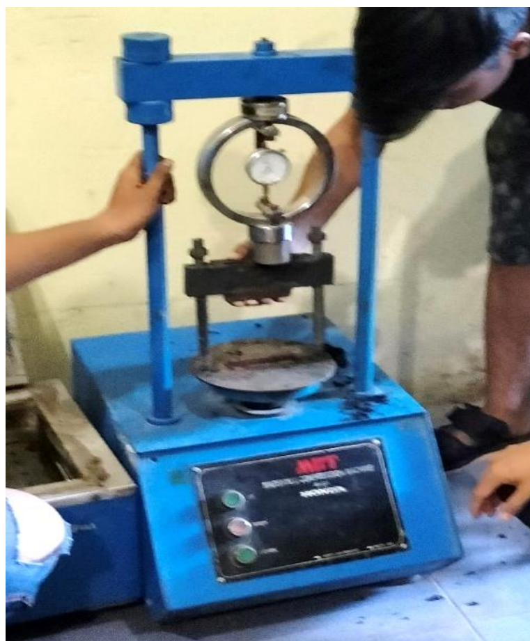
Figure 2: Set up stability and flow test layout
