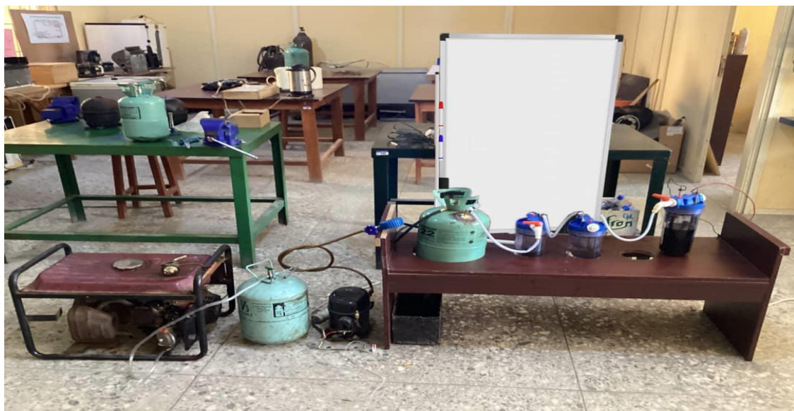
Figure 12: Set up of the electrolysis process of urine
