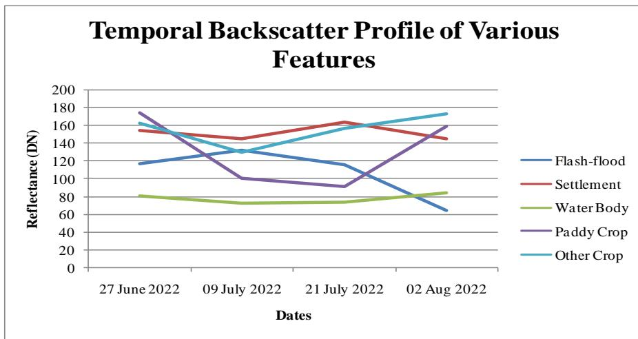
Figure 3: Backscatter profile of SAR data over various spatial features
