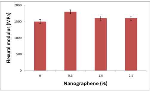
Fig 2: Nanographene loading vs. flexural modulus of FPF/HDPE nanocomposite
