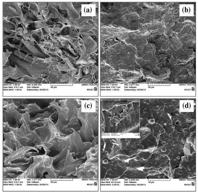
Fig 4: SEM images of composites containing 35 wt % FPF (a) 0 (b) 0.5 (c) 1.5 (d) 2.5% nanographene
