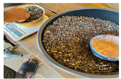
Plate 4: Recycled/crushed polyethylene (HDPE)
