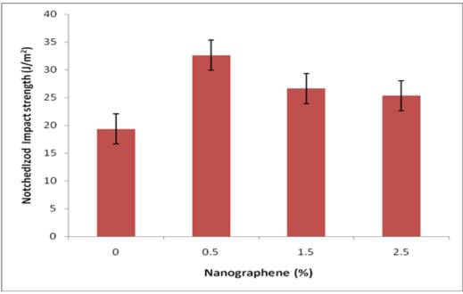
Fig 3: Nanographene loading vs. Impact strength of FPF/HDPE nanocomposite
