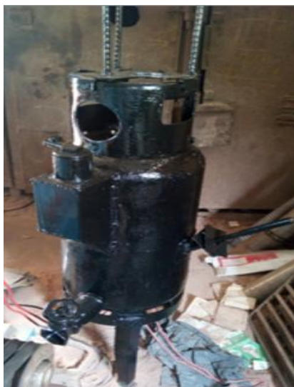
Fig-1: Fabricated Batch AD Digester
