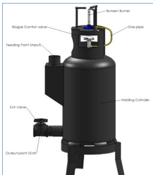
Fig-1: Isometric View of AD Batch Digester
