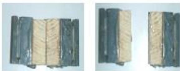
**Fig-3: Hot melt adhesive and middle breaks**
