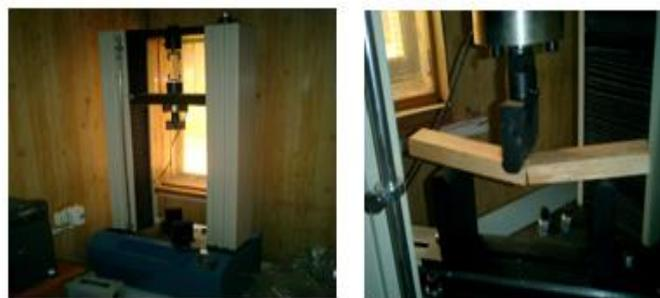
**Fig-2: "UTM" machine and ASTM D3930-8 test**
